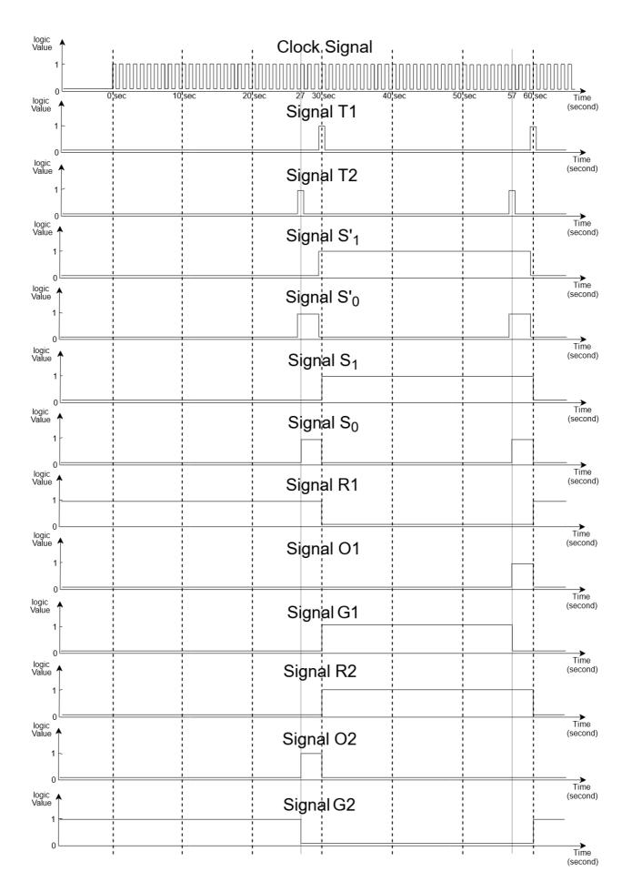
**Remark 1:** The frequency of the clock was not indicated in the exercise, but it can be deduced that the period cannot exceed 3 seconds, because the minimum signal change in the circuit is 3 seconds, that of the orange light. We chose 1 second as the period, therefore a frequency of 1 Hertz.
