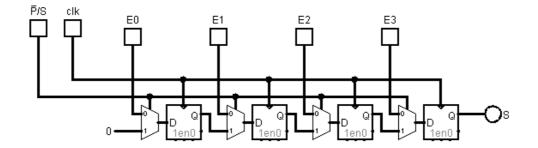
**Remark 1:** The  $\overline{P}/S$  (Parallel/Serial) control input allows to choose between, entering the 4 inputs in parallel, or shifting the values in a chain through the cells to output them in series on the S output.
