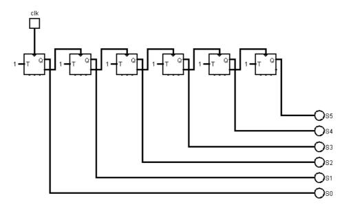
**Remark 4:** The Counter has the ability to oscillate its outputs by doubling the period for each output, which gives it the ability to be used very often as a frequency divider. For example, if you apply a frequency of 1 KHz to its clock, the first output will produce a signal of 500 Hz, the second of 250 Hz, the third of 125 Hz, and so on.
