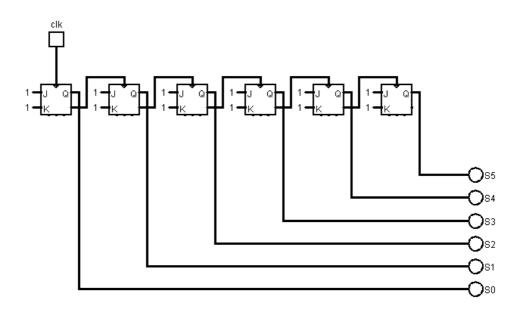
The 6-bit counter circuit based on T-FlipFlop :
