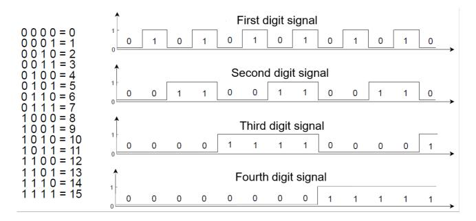
If we focus on a single column for a given digit, for example on the first digit. We can observe that it is a periodic signal identical to the clock signal. As well as for the second column, with the difference that it is double the first. And the third is also double the second, and so on and so forth. The signals of all its 4-bit digits are transcribed in the right part of the above figure.
