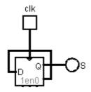
To make the signal of digit taking twice the period of the previous digit, we simply use the output of the previous digit as a clock for the current digit. As in the figure below. You note that in the figure we take the signal  $\overline{Q}$  instead of Q. Because by observing previous graph of the signals above, we notice that the digital signal really changes value during the Falling Edge of the previous digital signal. This forces us to use the inverse signal  $\overline{Q}$  instead of Q.
