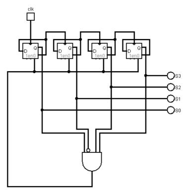
**Remark 3:** The Reset in this solution is supposed to be Asynchronous, if it was a Synchronous command the solution should be different.
