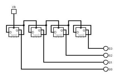
To limit the count to the value 12 (1100), it is wise to use the FlipFlip Reset command which will reset all the FlipFlops to 0 when the circuit detects that it has reached the limit. The limit in our case should be the value 13, the value just after 12, which should simply be detected by an AND gate. The Reset used here is Asynchronous, so it will reset the cell immediately after detecting the value 13. It practically instantaneous, the counter will never get enough time to hold the value 13.
